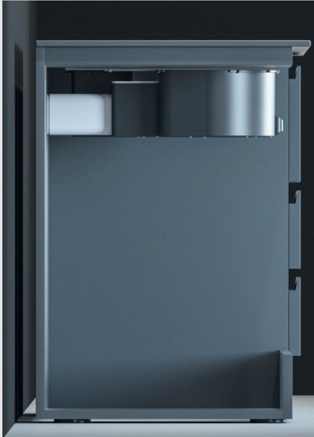
A carbon filter must be used with the Plug & Play kit (YT207.1001.91). Installation is made by connecting the adapter and flex pipe with tape. The clean air passing through the filter is discharged outside behind the counter.
