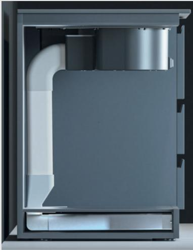
This installment can be performed with the code YT207.1001.89. First, the following cut should be made in order for the pipe to pass to baseboard on the counter top. Then the pipe should be placed and taped to each other, the orientation of the vent on the counter (front, rear, right or left) can be adjusted with flex pipe and the H6 vent slot is opened to the baseboard.
