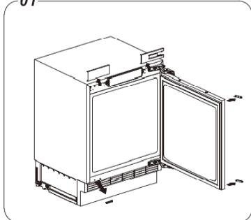
2. With the door closed, remove the screws on the outside of hinges. Open the hinges away from the door. With the hinge open undo the screws holding it to the cabinet. Be careful with the hinge, use a long shafted screwdriver if you have one.
