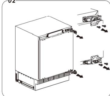
3. Turn the hinge over and place it on the diagonally opposite corner of the cabinet. Screw back in place. Repeat with the other hinge. Replace the door and re-attach the hinges. Check that the door is aligned horizontally and vertically and that the door seals are secure on all sides before finally tightening the hinge bracket screws.
