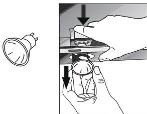
For replacing the halogen lamps, push downwards on the lamp holder from its behind, turn it a little bit counter-clockwise, and take it out downwards. Fig. 15
